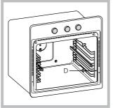
3. Secure the two frames with the guide rails using the holes provided on the oven walls (*see diagram*). The holes for the left frame are situated at the top, while the holes for the right frame are at the bottom.
